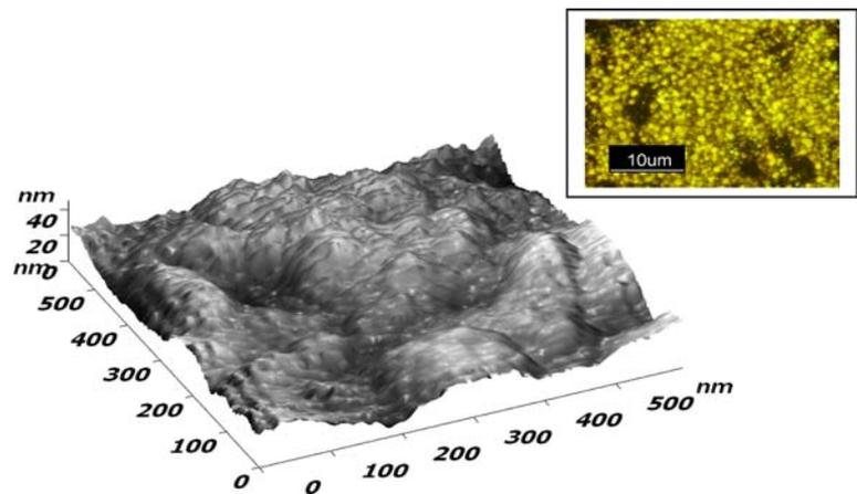
**Fig. 3** AFM image of anodized pure titanium surface, inset showing epifluorescence micrograph of similar oxide film
