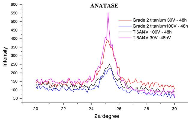
**Fig. 1** GIXRD results of grade 2 titanium and Ti6Al4V alloy surfaces anodized at 30 and 100 V for 48 h
