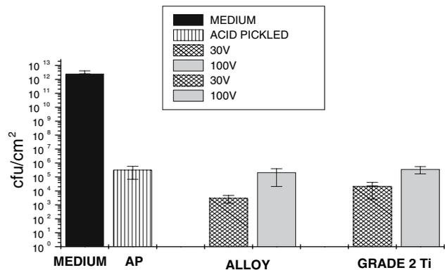
**Fig. 5** Total viable counts (TVC) of *Pseudomonas* spp. on anodized pure titanium and alloy surfaces under near-UV light illumination
